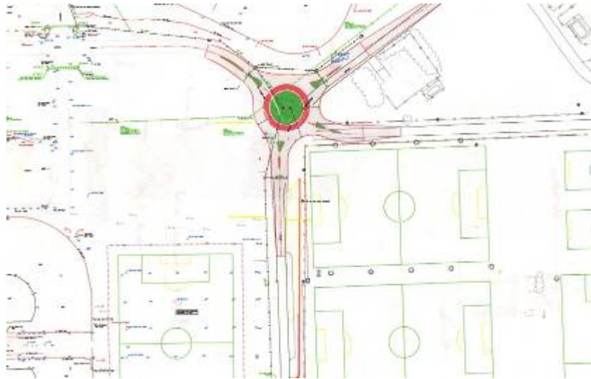
Figure 10: Engineers design of the rain garden in the center of the roundabout that will draw runoff from the surrounding athletic fields.
